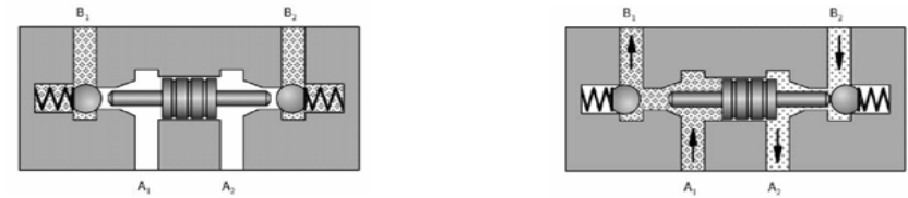
Piloted double non-return valve, closed Piloted double non-return valve, open
