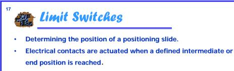
Limit switches can be connected up as N/O, N/C or changeover contacts.
